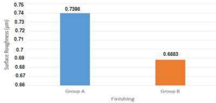
Figure 1. Surface roughness comparison between groups before the polishing procedure. Group A: Nanofilled composite resin Filtek Z350 XT, Group B: Nanohybrid composite resin Filtek Z250 XT, Finishing procedure using coarse type Sof-Lex XT Disc
