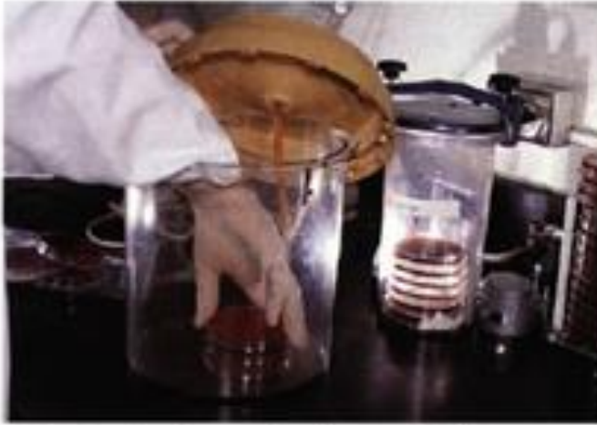
3-31 Prereduced anaerobic plates can be held in an anaerobic holding jar for a short time before and after inoculation.
