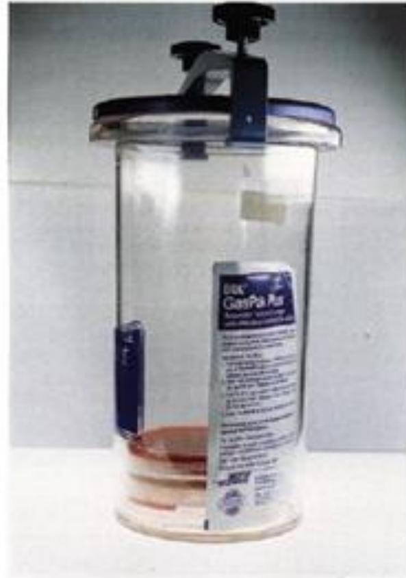
3-31 Prereduced anaerobic plates can be held in an anaerobic holding jar for a short time before and after inoculation.
