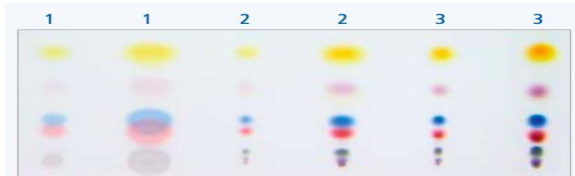
Developed plate after contact application of spots
